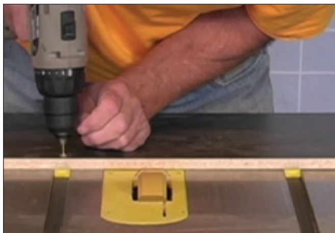
Drill holes in all four corners to attach the miter tracks to the base
